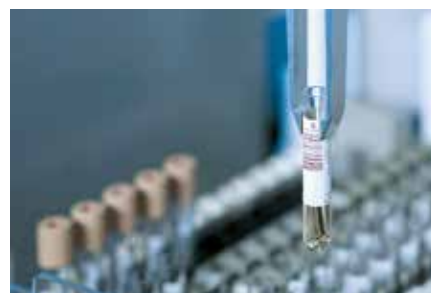
Tube transfer e. g. to a balance by the Pick and Place arm.
