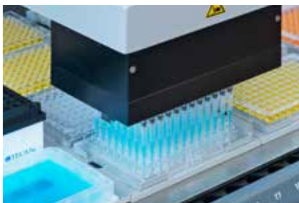
The MultiChannel Arm 96 pipetting with 96 channels in parallel speeding up your assays.
