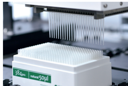
Multiple Channel Arm picking up one row of 24 50 µl tips
