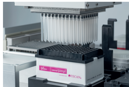
Multiple Channel Arm picking up 96 500 µl disposable tips
