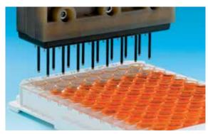
Eight- or 16-way manifold for ELISAs and cell-based assays, allowing simultaneous washing of eight or 16 wells
