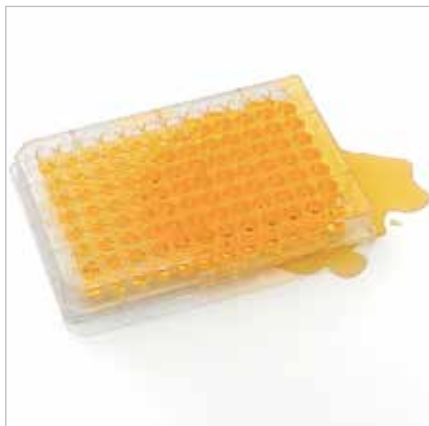
Spilling of plate caused by clogged needles
